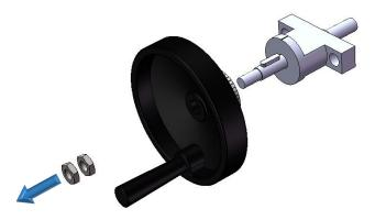
3. Remove the key from the lead screw.
