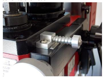
7. Verify that the spindle lock engages and releases smoothly with no binding.
