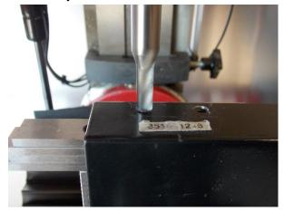
5. Install the spindle lock with the included screws, lock washers and nuts to the feed cover.
